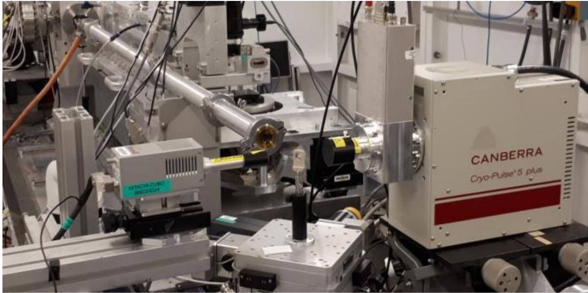
**Figure 1** - Picture of a single channel detector prototype under beamline test on BM23 at ESRF
