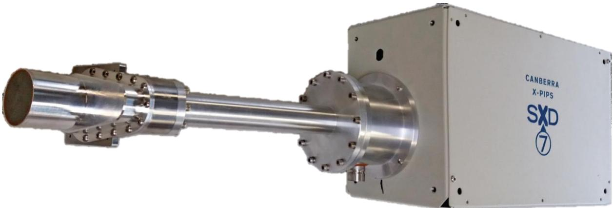
**Figure 2** – 7x 50 mm<sup>2</sup> SDD array in close packed configuration with 1.4W Cryo-Pulse electrically refrigerated cryostat
